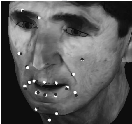
Figure 12.15 Illustrates placement of the points for the new model of WM, which corresponds to Baldi's wireframe morphed into the shape of DWM. These dark points are placed 3mm (4mm for the chin point) off the synthetic surface and the placements of the corresponding measured OPTORAK points are given in white.
