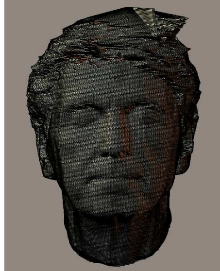
Figure 3. High-resolution polygon mesh obtained from the Cyberware laser scan.
