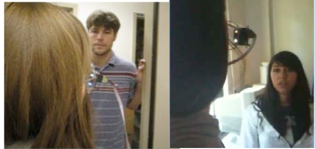
Figure 1. Two illustrations of the iGlasses in use. The wearer sees the talker in central vision as well as the cues shown on LEDs in the periphery.
